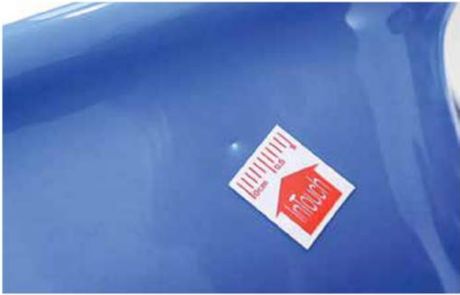
Figure 4. Example of a pinhole defect in a finished ceramic product.
